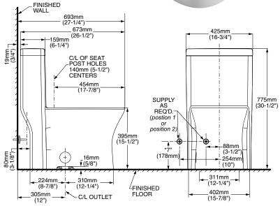
IMPORTANT: Water supply on the wall is required at 3-1/2" (88mm) or 10" (254mm) from centerline of the toilet (see rough-in). First suggested position is hidden behind the toilet. The geometry of the toilet gives space for this installation. The second suggested position is next to the toilet. Between these two positions, the space for the supply between wall and toilet is limited to 3-1/8" (80mm). In this case, check your supply and hose dimensions.
